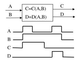
I/O No clock-delayed constraints
