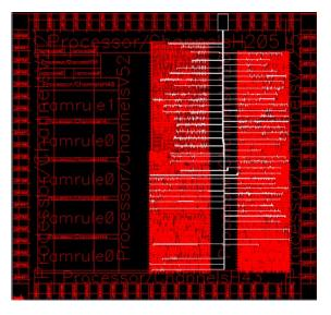
If the layout is completed, the wire lengths and thus the propagation delays due to parasitics will be known. The design can be simulated on gate level netlist added with propagation delays, after *backannotation*, and, consequently, *the timing behavior of the entire circuit can be validated*.
